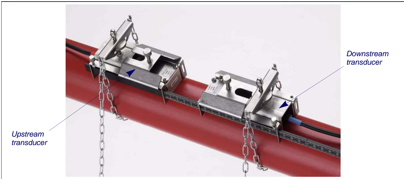
Figure 2.4 Completed transducer assembly
