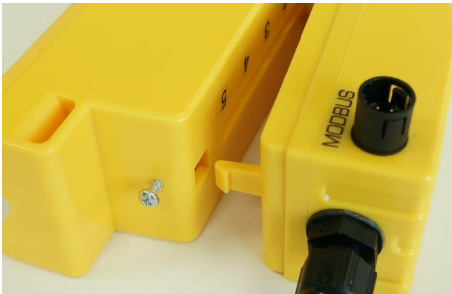
Figure 24 Separating Sensor Assembly and Electronics Module
