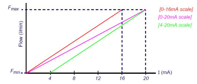
To calculate the flow rate (l/min) for a measured current (mA) then:
