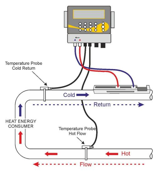
Figure 19 UF3300 Heat Meter Temperature Probe Positioning (Heater system)
