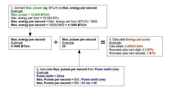
How to calculate a suitable Energy per pulse value from Maximum power and Pulse width (Metric)
