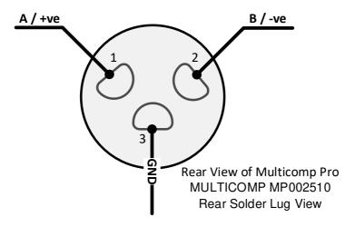
Figure 22 - UF3300 Modbus Plug Connections
