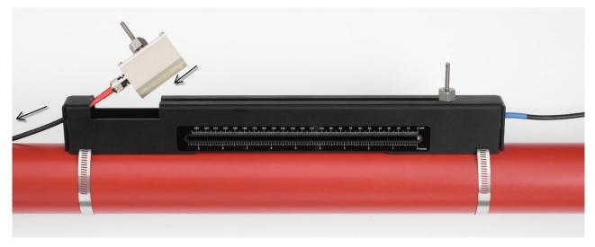
Figure 15 Installing upstream transducer (red)
