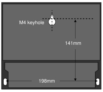
Figure 7 UF3300 mounting dimensions
