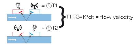
The UX5000 HazFlow is an ATEX certified, clamp on ultrasonic flow meter that accurately measures liquid flow within a closed pipe. Installation is simple and rapid and requires no process downtime or shutdowns. Pipes are not cut or modified in any way, the installation is completely non-invasive but the flow monitoring is accurate and reliable.
