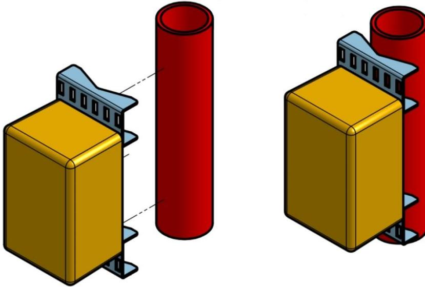
Figure 9: RMU: mounting to a vertical pipe
