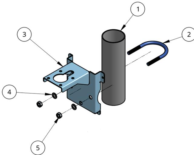
Figure 8: Pipe-mounting the DCSIU
