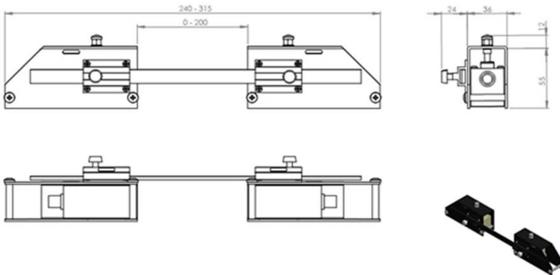
The sensor bracket assembly is configured for reflex (2 path) operation. For direct (1 path) operation the guide rail will not be used.
