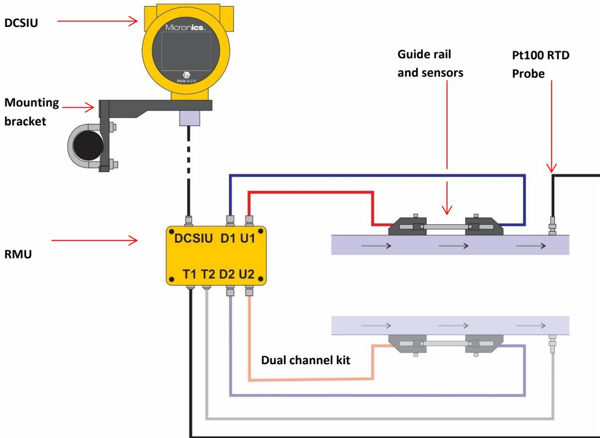
Figure 3: UX5000 system configuration
